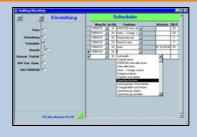
· Scheduler for time controlled remote read-out of the MAVOLOG 10 with the help of METRAwin 10 via RS 485 interface, modem or Ethernet using a slave PC as a gateway
