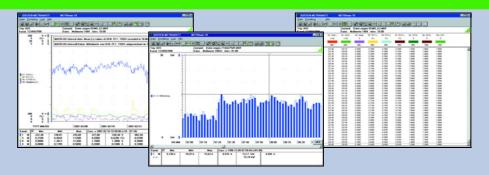
**Event data** read out from one or several MAVALOGs are listed in the order in which they occurred and can be printed out in report form. In the event of voltage dips, interruptions or swells, these are displayed in a Y-T diagram and can be analyzed with the cursors.
